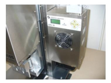
Because of the large number of existing plastic materials and their shapes is neccessary tested suitability of usage ultrasonic welding tool for concrete aplication. When thinner materials is welded in addition to set duration of weld, may also be needed to reduce output power of ultrasonic generator.
